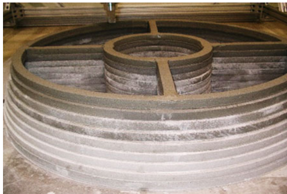
Fig. 1 3D-printed concrete element using CC technology (Davalab et al., 2018)
