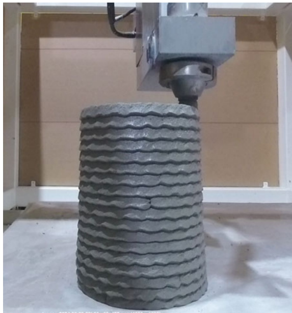
Fig. 4 3D printing of high-volume fly ash mortar with nanoclay inclusion (author's original) (Panda et al., 2019b)
