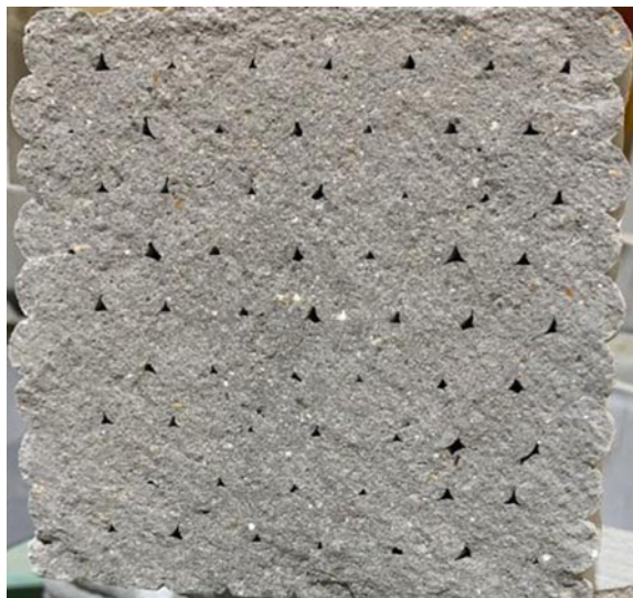
Fig. 6 Voids in 3D-printed concrete at NTU Singapore (author's original)
