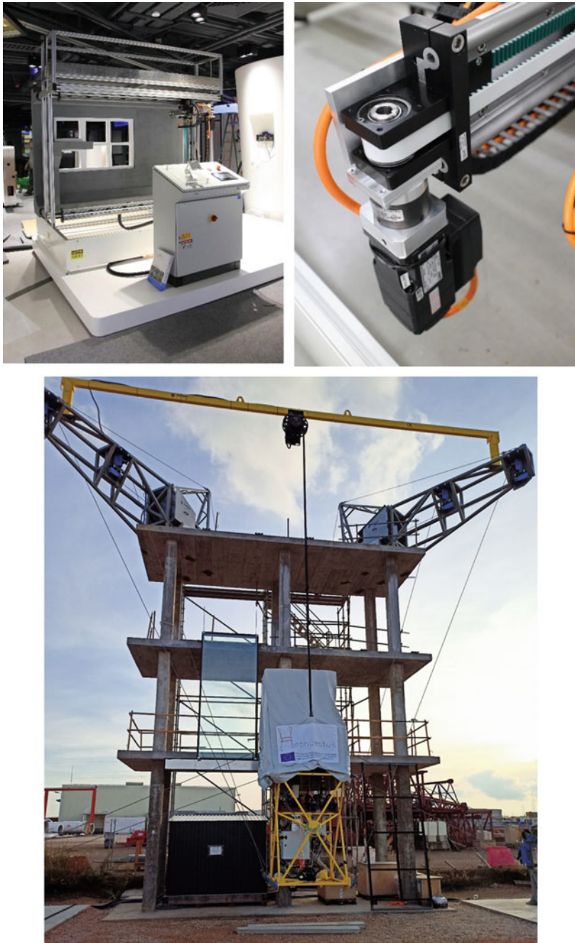
Fig. 13 Top left and right: prototype of the CIC robot ( photo R. Hu ); bottom: prototype developed and tested in the HAEPHAESTUS project in Madrid, Spain ( photo K. Iturralde )
