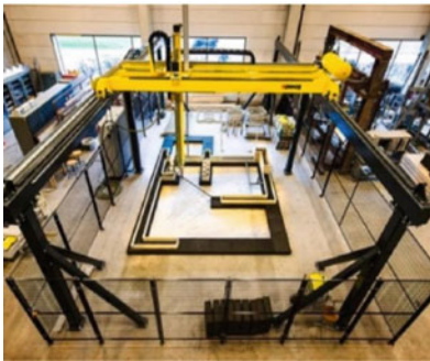
(A) Gantry C3DP system
