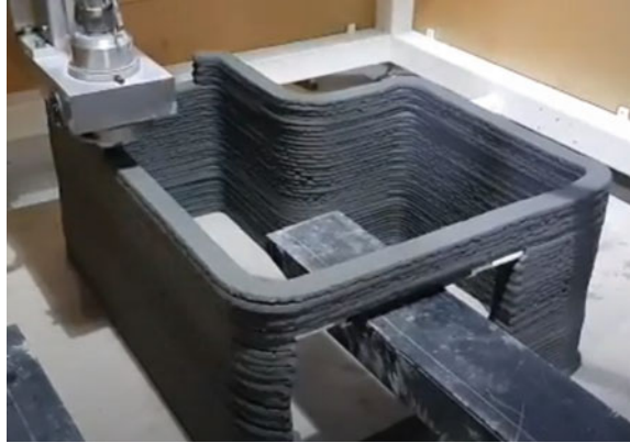
Fig. 3 Additive manufacturing of overhanging concrete structures at NTU Singapore (author's original)
