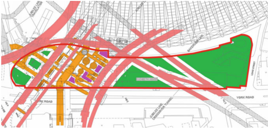
Fig. 18 Piled foundation zones
