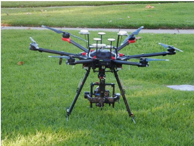
Fig. 3 Survey drone with cameras and LiDAR. Source https://live.staticflickr.com/851/41994685850_73358db510_b.jpg . Available through the creative commons licence
