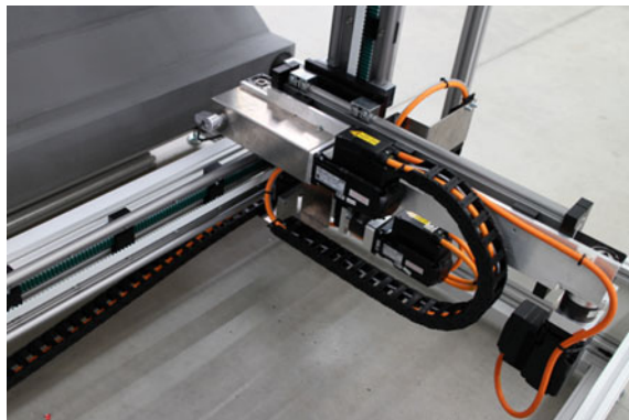
Fig. 10 In the context of the facade processing robot developed for CIC, the operation sequence and the composition of the robot were simplified in previous steps that allows the robot to be built fully from standard linear axes and drives ( photo R. Hu)
