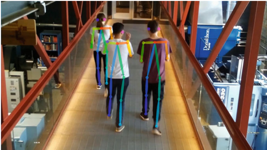
Fig. 8 Extracted skeletons overlaid onto video of people crossing the Pier 9 bridge (author’s original)
