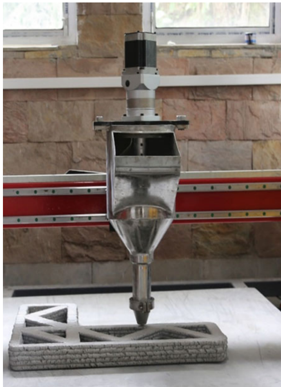
Fig. 2 Extruder-based 3D concrete printing (author's original)
