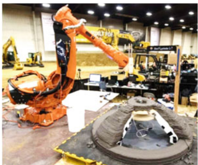
(C) Modified articulated robot used for C3DP
