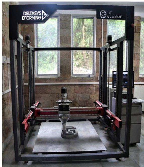
Fig. 1 3D concrete printer facility at Indian Institute of Technology Guwahati, India. (author’s original)
