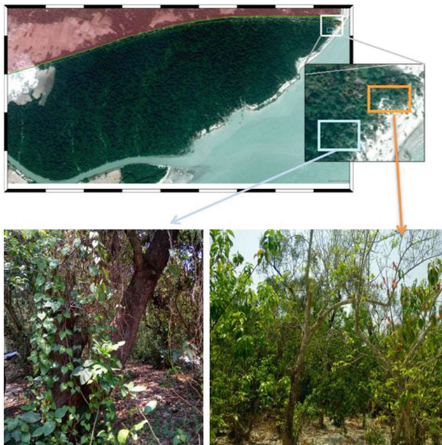
Fig. 12 Manning's roughness calculation sample area (a) Section-1: less dense area (represented by orange box) and another one is (b) Section-2: comparatively denser area (represented by the blue box)
