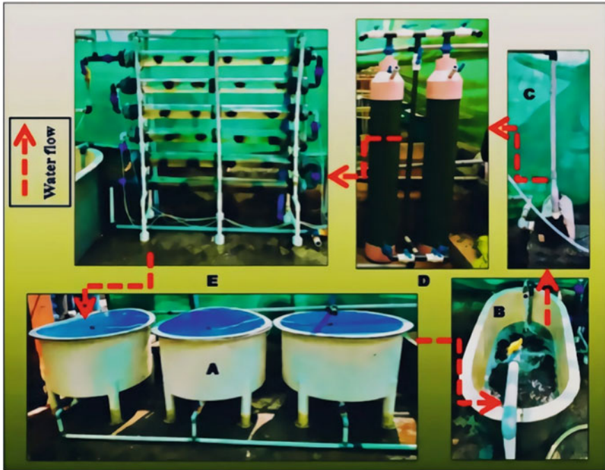
Fig. 34.12 RAS with tubing bioreactor a shrimp culture tanks, b sump, c pump, d pressure sand filter, e seaweed bioreactor. Red color arrow indicates the flow cycle of water in the system
