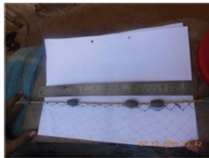
e. Joining of selvedge meshes and attachment of sinkers
