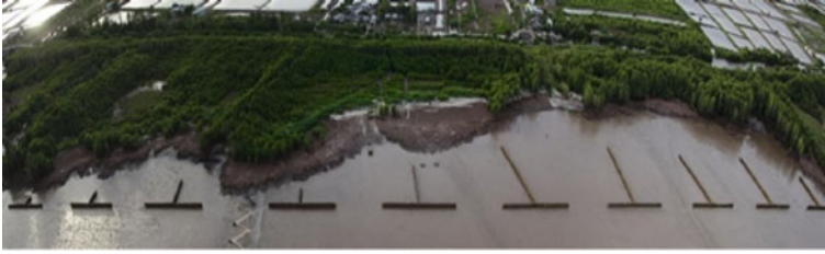
Fig. 64.10 Bamboo T-fence in combination with mangrove forest for coastal cyclone and flood management in Bac Lieu Vietnam (Dao et al. 2018)
