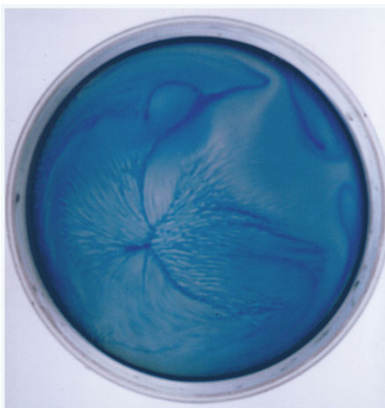
Fig. 15.1 Structure formation in the blue miracle in a Petri dish after 2 min. The glucose gel was produced from 20 ml glucose 2 M to 10 ml NaOH 2 M and then covered with 20 ml methylene blue 10^{-3} M. The resulting layer height was approx. 9 mm. (Photo: S. Huth, N. Tobias and P.J. Plath)
