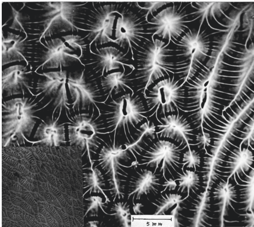
Fig. 10.16 Collective behavior of ROWI; large picture: system air/CS 2 at 45 °C; small picture bottom left: system butanol/5% CuCl 2 + water
