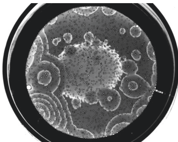
Fig. 1.1 Waves and phase waves at the Belousov–Shabotinsky reaction (BZR) in a Petri dish. Both are purely chemical waves. They move with quite different velocities and shape of their fronts (photo: P. J. Plath). With the discovery of oscillations and waves in the BZR, the ideas of synergetics by Hermann Haken became popular in chemistry too
