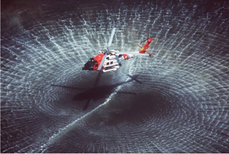
Fig. 11.3 Foam streaks by the radially ordered wind of a helicopter at the sea (downwash under helicopter); published in the Public Domain by the Defense Media Activity Enterprise Customer Services (DVIDS) of the US Department of Defense (DoD) [9]
