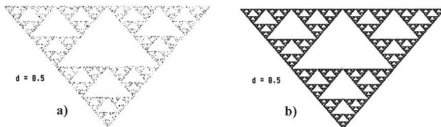
Fig. 6.7 Sierpinsky gaskets generated by an iterative random process. The division ratio between the randomly selected attractive corner point and the iterated, wandering point is d = 0.5 ; a with a low number of iterations; b with a high number of iterations, for which the set of iterated points has come very close to its attractor
