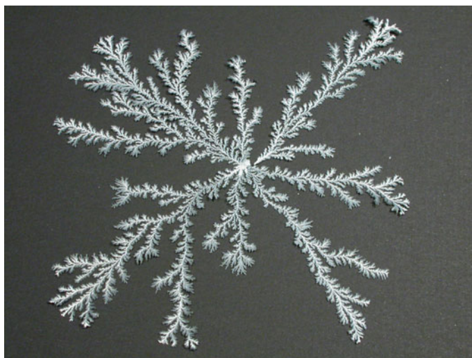
Fig. 5.1 Growth of the metal zinc-tree in a Petri dish at a voltage of 6 V. The 2 N zinc sulfate solution was covered with a layer of n-butyl acetate. For this picture the zinc tree has been removed from the Petri dish and placed and dried on a grey cardboard. ( Photo taken by Thomas Rabbow )
