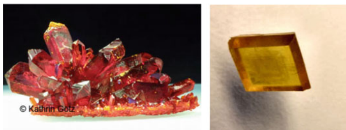
Fig. 4.21 Left potassium ferricyanide III \text{K}_3[\text{Fe}^{\text{III}}(\text{CN})_6] ; right potassium ferricyanide II \text{K}_4[\text{Fe}^{\text{II}}(\text{CN})_6] 17 mm × 15 mm und 9 mm; (Photos are made by Kathrin Götz [12] and Hubert [13])
