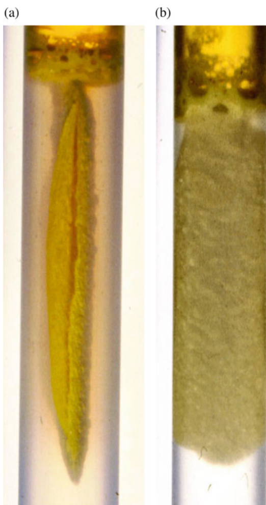
Fig. 3.19 Example for the new precipitation pattern in a test tube: tongues-formation: inner electrolyte 0,21 M \text{Pb}(\text{NO}_3)_2 ; external electrolyte: saturated potassium chromate \text{K}_2\text{CrO}_4 solution; maturing time of the gel < 10 h. a side view: splitting of the tongue, b frontal view: the same tongue viewed from a perpendicular position. (Photo: C. Müller, P.J. Plath, 1993)
