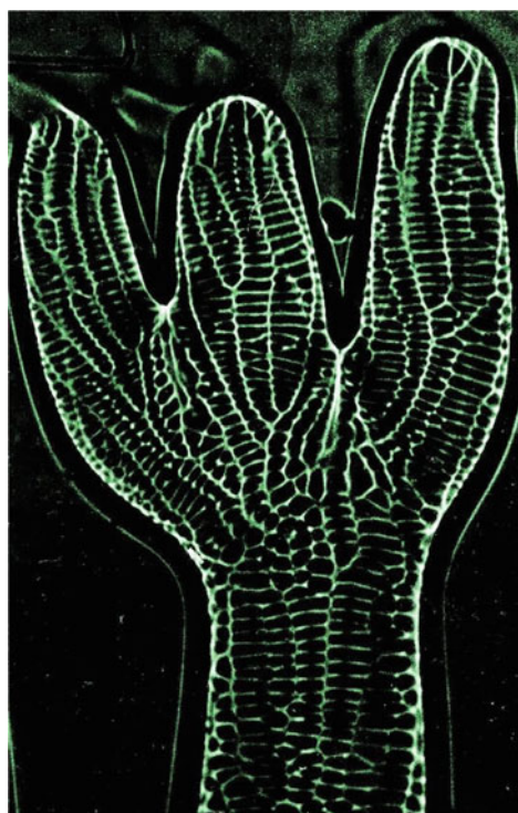
Fig. 11.1 Coupling of meniscus flow and Marangoni instability. The roll cell boundaries are displayed
