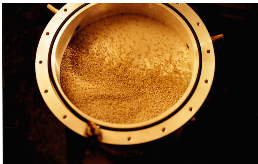
Fig. 8.1 Vibrated granular quartz (Rutile) layer (2 mm) at 66.4 Hz and an acceleration b \approx 10.1 g. The wave is moving uphill the faraday heap which has been formed at the wall of the vessel (photo: P.J. Plath).
