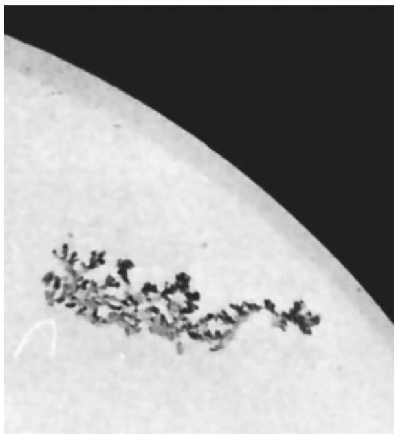
Fig. 5.16 Disconnected Zinc particle moving freely towards the ring anode via fractal growing at the front side and dissolving in its rear. Experiment with 14 V at 1:29 min after starting
