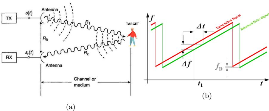
**Fig. 1.** (a) Typical radar working principle using reflected RF signal (b) FMCW radar waveform.
