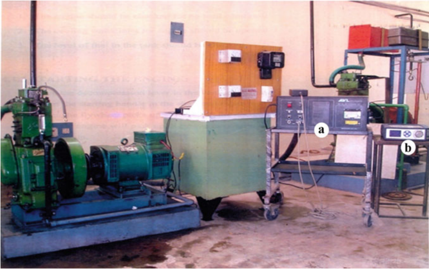
Fig. 15.2 Experimental engine a AVL smoke meter, b AVL DIGAS analyzer
