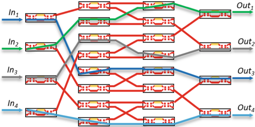
Fig. 3. Schematic of a proposed example 4 \times 4 dilated Banyan network. (Color figure online)
