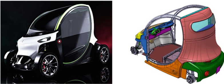
Fig. 1. Render and model of the present electric micro-car in linen bio-composite. (Color figure online)
