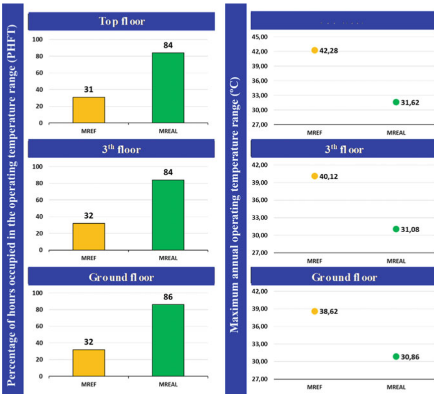
Fig. 13 Numerical results for evaluating the minimum level of performance of the social building
