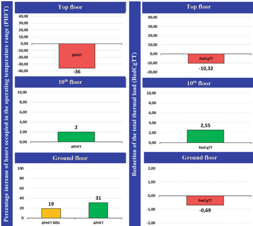
Fig. 16 Numerical results for evaluating the intermediate and superior level of performance of the high standard building
