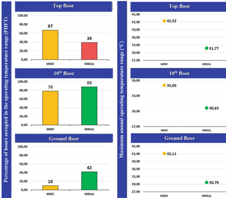
Fig. 15 Numerical results for evaluating the minimum level of performance of the high standard building
