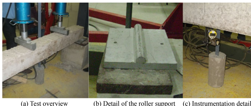
Fig. 3 Four-point beams tests
