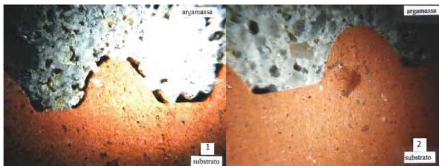
Fig. 1 Aspect of the interface region between mortar with different proportions of cement and lime, and base in ceramic brick (Carasek, 1996)
