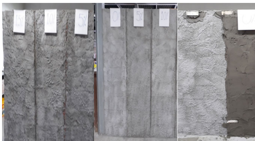
Fig. 7 Concrete block base with a lime solution and plaster application
