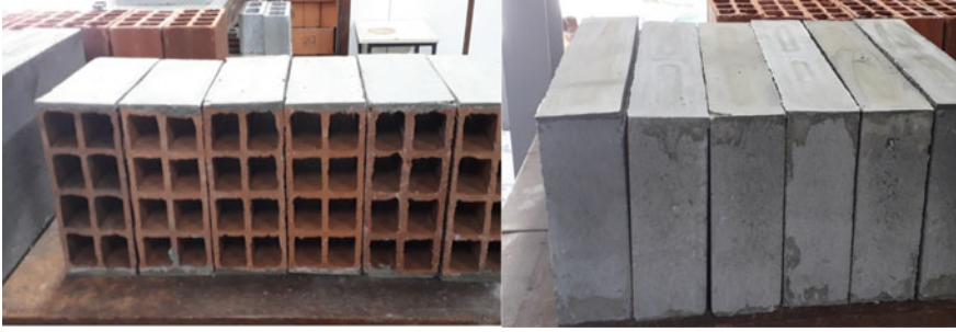
Fig. 13 Ceramic and concrete blocks used
