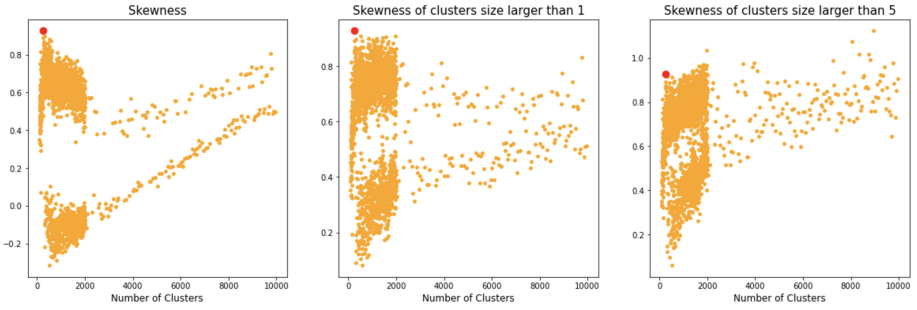
Fig. 2. Skewness over spherical k-means clusters: over all clusters (left), over clusters of size great than 1 (center), and over clusters of size greater than 5 (right).
