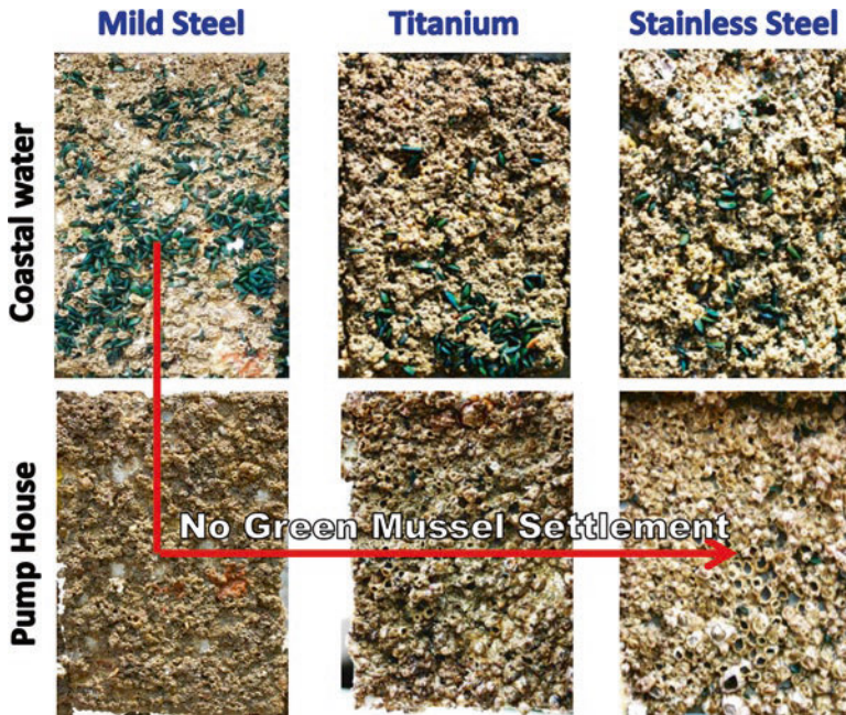
Fig. 7 Biofouling community on test coupons in kalpakkam coastal waters and at the pump house of MAPS
