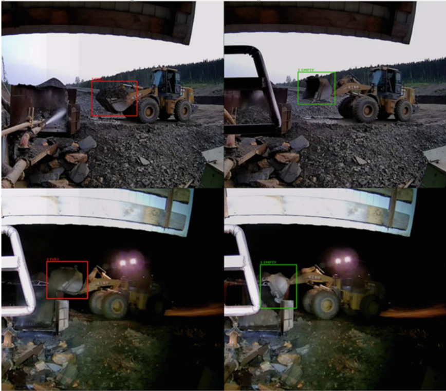
Fig. 6 Example of marking material for counting front loader buckets, where the top row is daytime and the bottom row is nighttime
