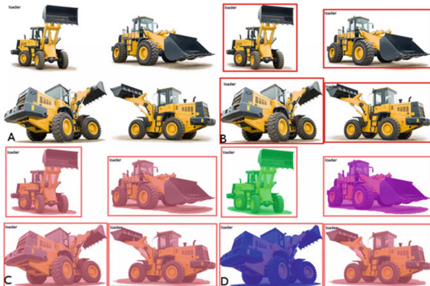
Fig. 2 An example of performing computer vision tasks, where a —the results of the classification task, b —the results of object detection, c —the results of the semantic segmentation task, d —the results of the instance segmentation task
