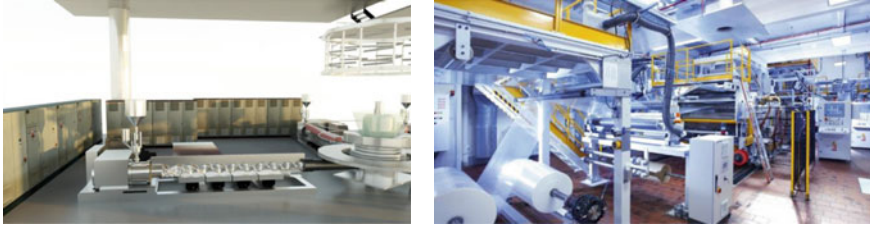
Fig. 1 Extrusion and calendrer lines for film materials production
