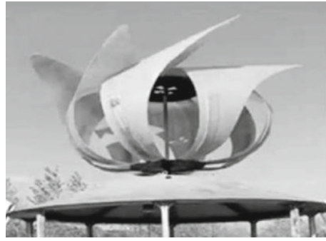
b) greater power WP testing P_2 = 1,2kW (at a nominal wind speed of 7 m/s)
