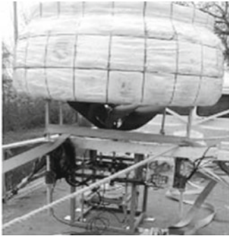
a) low power WP testing P_1 = 0,2kW (at a nominal wind speed of 7 m/s) on a car platform
