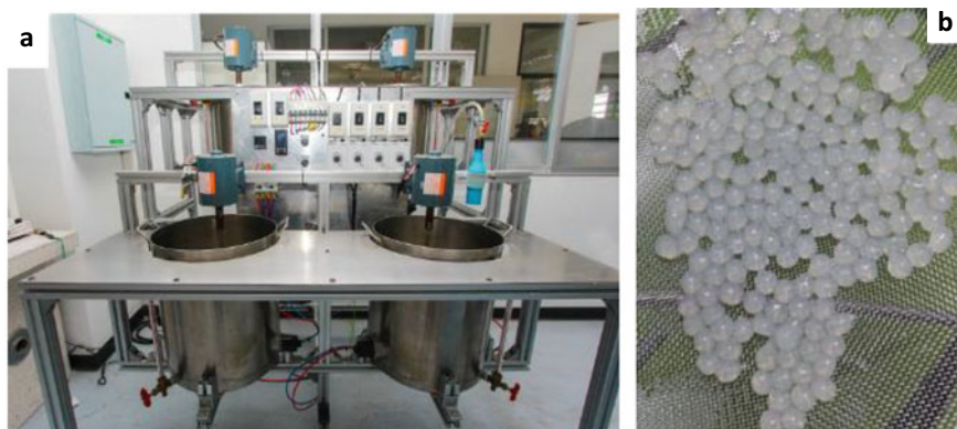
Fig. 2.8 a Digital image of prototype machine for manufacturing of hydrogel beads and b the produced chitosan hydrogel beads. Reproduced with permission from [44], Copyright 2021, Elsevier Science Ltd.
