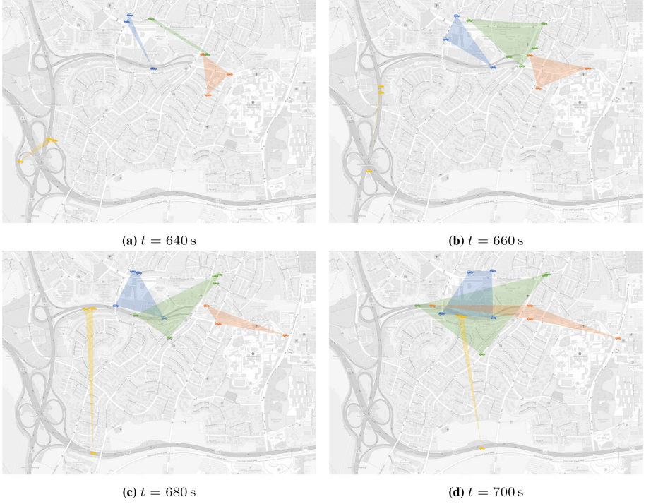
Fig. 10. Extract from the Vehicle movements and group formations for different simulation times t and \Delta t_{G,c} = 20 s, \Delta t_{G,v} = 60 s, \Delta t_{G,i} = 80 s, and \Delta t_{M,b} = 1 s.
