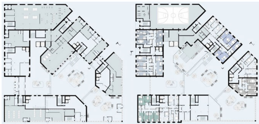
Fig. 12 First and second floor plans. In the central part of the building, there is an all-season courtyard with public infrastructure. The pilot project of a public-residential complex for the Far North (Nadym city). An architect is E. Denshchik, leaders are A. Merenkov, N. Lamekhova
