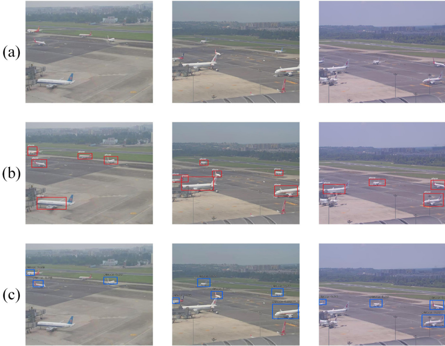
Fig. 7. Comparison of proposed method with Faster RCNN: (a) Current frame (b) Faster RCNN (c) AMORnet
