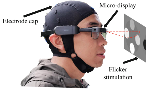
Fig. 2. The equipments that the user needs to wear when controlling the aircraft.
