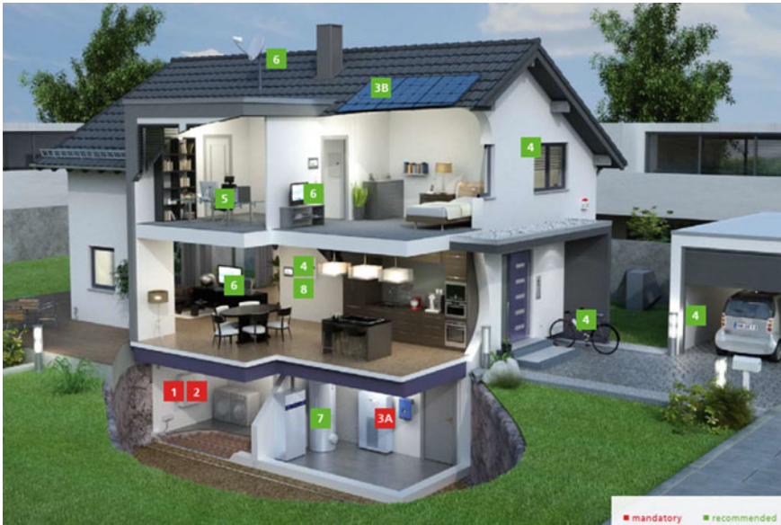
Fig. 3.2 Lightning protection of a single-family house without external lightning protection. Credit: DEHN, with permission
