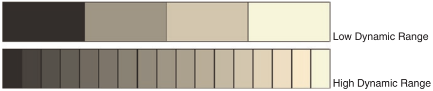
Fig. 3.14 Demonstrates the contrast between high and low dynamic range [with permission from SonoSite]
