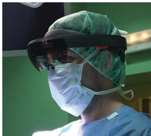
Fig. 6.12 A head-mounted display which is utilized in the augmented reality. Reproduced with permission from [60]
