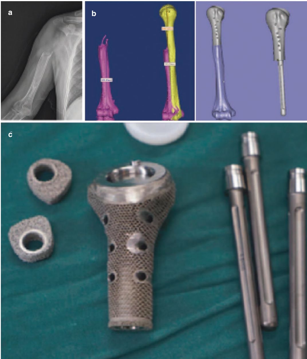
Fig. 22.2 Preoperative data and design and manufacture of prosthesis: (a) bone defect observation, (b) prosthesis design, (c) the shoulder parts manufactured with EBM technique [22]
