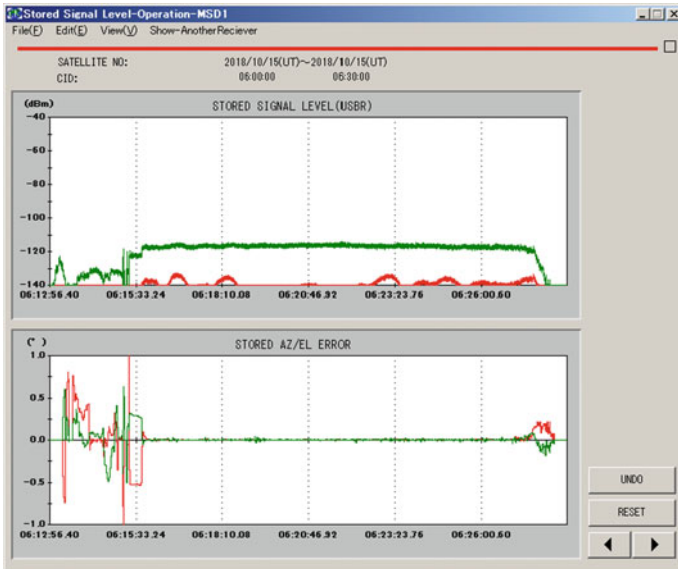
Fig. 2 AGC Level (RHC/LHC) and antenna pointing Az/El error profile
