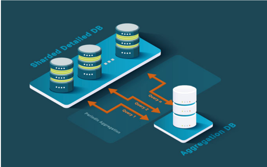
Fig. 3.7 Detail-aggregate view splitting architectural pattern
