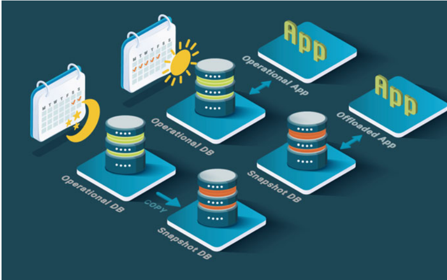
Fig. 3.4 Operational database off-loading architectural pattern
