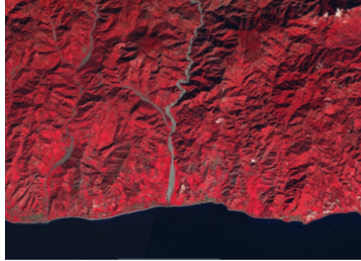
Fig. 2. Sentinel 2 false color image (RGB = bands 8, 4, 3) of a subset of the province of Reggio Calabria including the study area.
