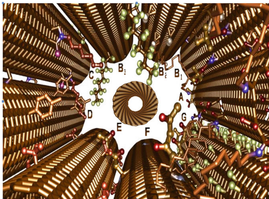
Fig. 4 Different methods for the covalent attachment of functionalities to the SWCNT sidewall carbon atoms. a Formation of amides or esters with the carboxylic acid groups of oxidized SWCNTs. b addition of nitrenes (B1), carbenes (B2), and radicals (B3). c [2 + 3] cycloaddition of azomethine ylides. d Electrochemical functionalization with diazonium salts e nucleophilic attack of Lithium alkyls. f Mannich-type reaction with N-doped single-walled carbon nanotubes. g Fluorination (Reproduced with permission from Ref. [16])
