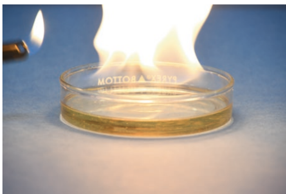
Fig. 3.3 Gasoline vapors ignited by an ignition source \sim 10\text{ cm} away from the liquid
