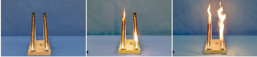
Fig. 3.22 Small scale demonstration of the influence of slope in a fire spreading uphill versus downhill (left) two identical channels filled with fire paste, (center) ignition at top and bottom 0 s, (right) flame spread downwards has only involved 1/10th of the fuel, while spread upwards has involved all of the fuel 20 s
