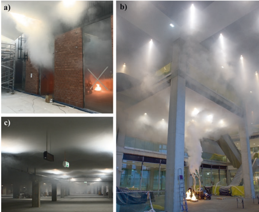
Fig. 4.2 Smoke flow phenomena inside buildings. (a) door flows in a compartment fire; (b) complex spill plume; (c) homogenous smoke layer in a large open-plan compartment. All pictures were taken during “hot-smoke tests”
