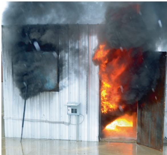
Fig. 3.20 Fully involved enclosure fire
