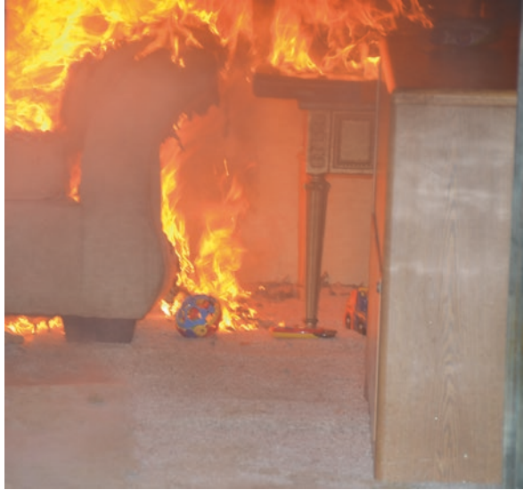
Fig. 3.19 Radiant ignition of fuels throughout the compartment beginning the transition to a fully involved enclosure fire
