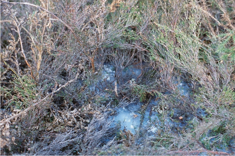
Fig. 8.2 Superabsorbent polymer (short-term FFC) applied with ground equipment 20 h before to create a chemical fire-break
