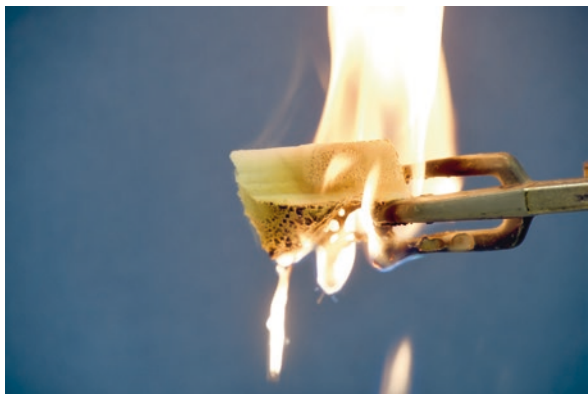
Fig. 3.8 Polyurethane foam ignited and burning
