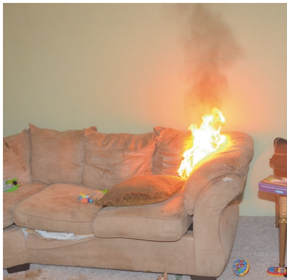
Fig. 3.15 Ignition of a couch inside an enclosure
