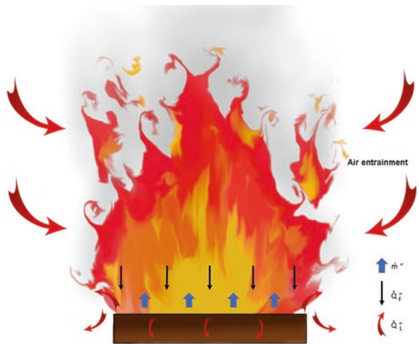
Fig. 3.9 Schematic representation of a burning surface, showing the heat and mass transfer process (illustration by Jennifer Taliaferro)
