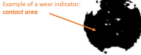
Fig. 8. Example of an electrode face imprint and identification of a target variable
