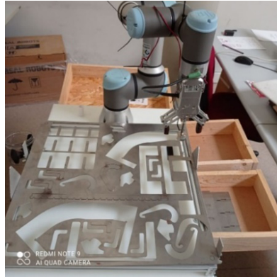
Fig. 7. Real case workcell with the automated detaching application.
