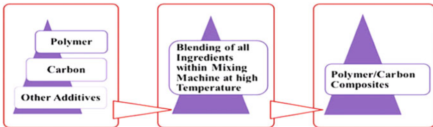
Fig. 2 Representative diagram of the steps of Melt blending [20]
