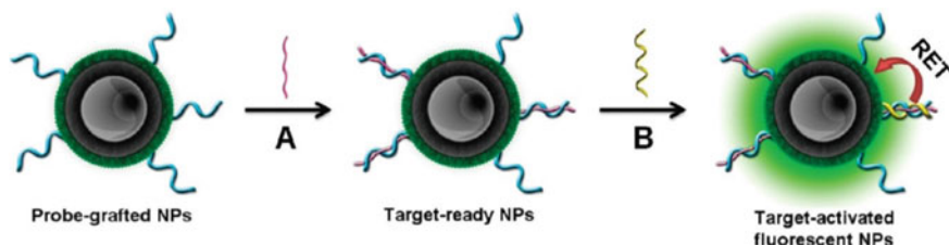
Fig. 21 Principle of DNA detection on fluorescent multilayer Core-shell Nanoparticles: A Target ready NPs are prepared by complexing ssDNA probe-grafted NPs with polymer transducer, B hybridization of target DNA with ssDNA probes activates the polymer transducer as energy donor toward dye doped silica shell and excitation at 410 nm generates fluorescence emission by acceptor molecules at 550 nm. Reprinted with permission from Ref [141] (A. G. Bracamonte-D. Boudreau et al.). Copyright 2011 ACS NANO, ACS
