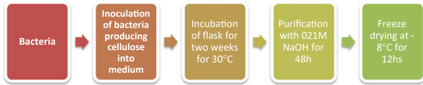
Fig. 6 The methods of producing cellulose by some types of bacteria
