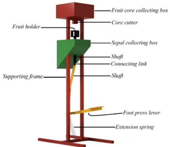
Fig. 3 Layout of foot operated MCC with detailed parts
