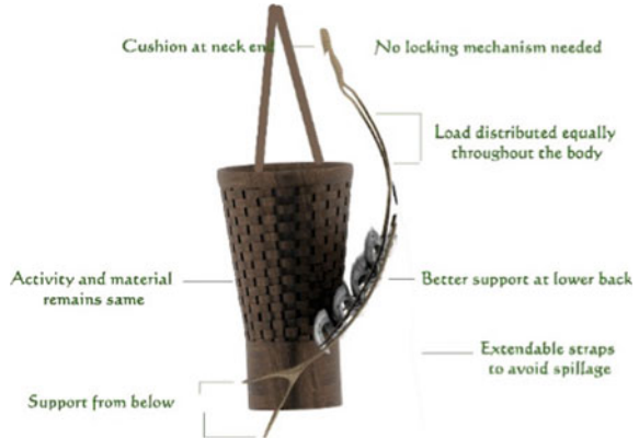
Fig. 8 Side view image showing details of the additional support strap with basket
