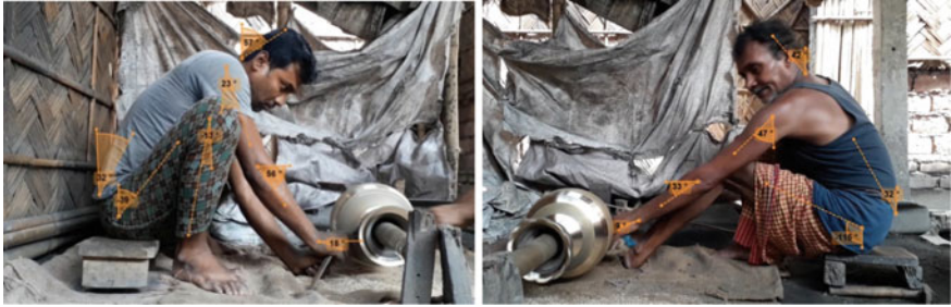
Fig. 4 The joint angle detection for handcrafted Kalash polishing
