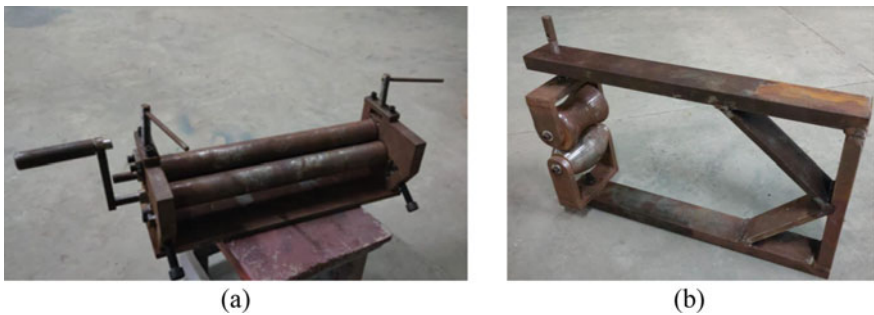
Fig. 6 a Prototype of sheet bending tool, b prototype of shaping tool
