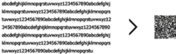
Fig. 3 A QR (Quick Response) code symbol of the size that can encode 300 alphanumeric characters. Source https://www.qrcode.com/en/ [1, 3]
