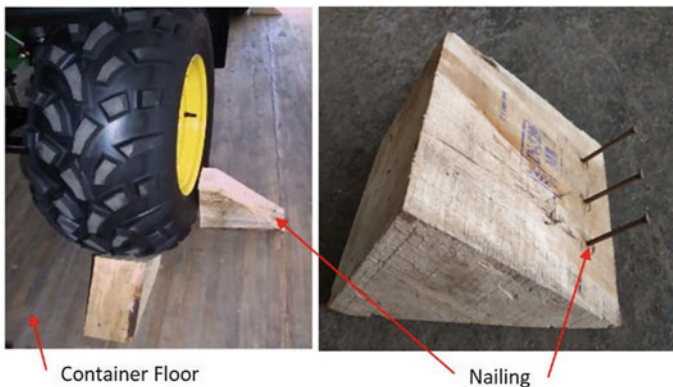
Fig. 1 Product secured using wooden block and nails
