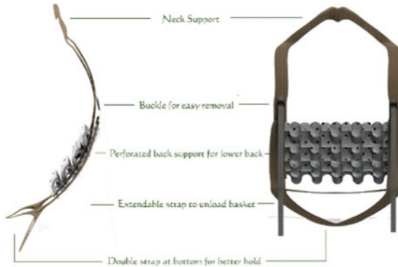
Fig. 9 Image showing details of the additional support strap
