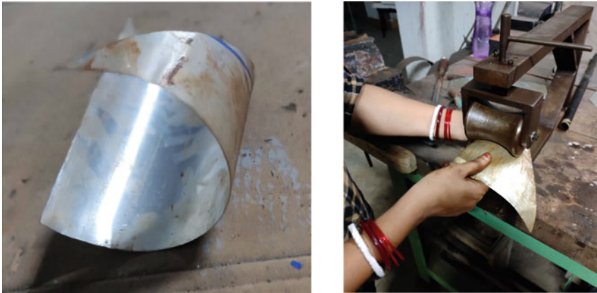
Fig. 7 Images of bend sheet and shaping operation of sheet respectively
