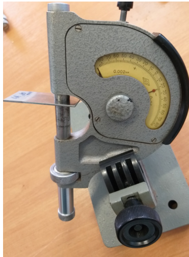
Fig. 5. Measuring the thickness of the sample-plate
