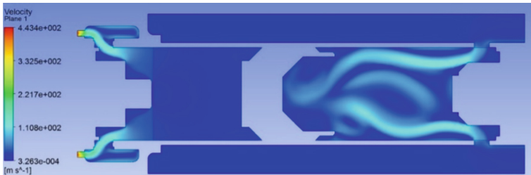
Fig. 9. Gas flows in the pneumo-impulse hammer channels
