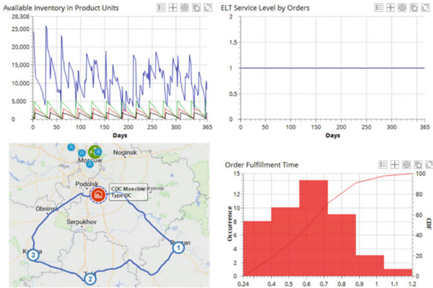
Fig. 5 Service and inventory levels after safety stock optimization and introducing milk runs
