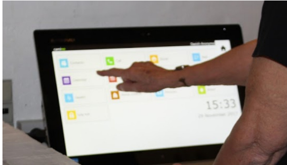
Fig. 1. The CARIOT+ CareCoach platform running on a touch screen device in the home of an end-user with the CAMINO user interface. The screen is an “always on device”, which allows the user easy access for launching apps and getting information. A pattern adapted by several commercial AAL vendors, and used in more than 10,000 deployments.
