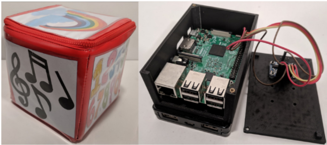
Fig. 1. Left: dice. Right: sensors placed inside the dice
