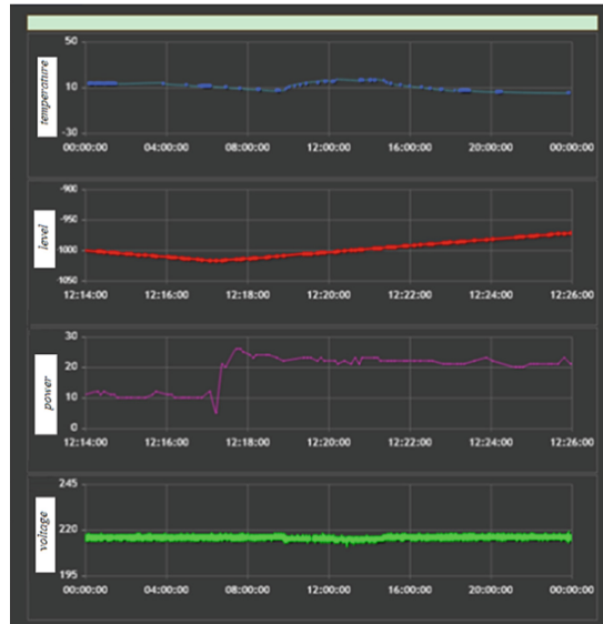
Fig. 6. Scraper descent from the top position to the bottom position and beginning of lifting.
