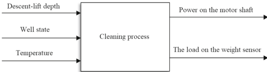
Fig. 3. Structure of the well cleaning process model.
