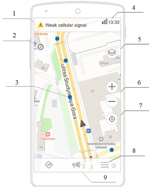
Fig. 7. The graphical interface of the software: 1 - messages and system alerts, 2 - reset the orientation of the map, 3 - vehicles, 4 - mobile network status, 5 - map display mode, 6 - map scaling, 7 - camera linking, 8 - settings, 9 - broadcast alerts.
