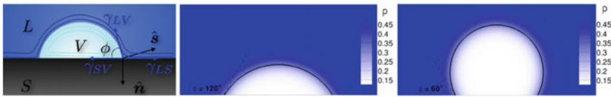
Fig. 3 Left: density field sketch for a bubble deposited over a solid surface. Center: Equilibrium configuration of bubble in contact with a lyophobic wall. Right: Equilibrium configuration of bubble in contact with a lyophilic wall. Reproduced from [7]
