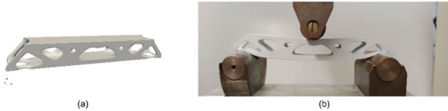
Fig. 5 From numerical results to 3D printed structure: a three-dimensional virtual model of the optimized geometry as obtained from TO solution, b experimental test of the 3D printed structure
