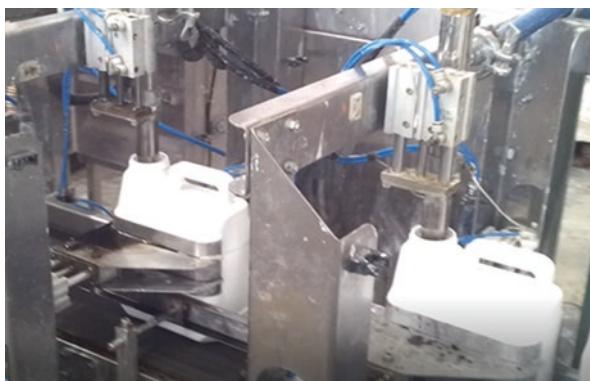
Fig. 32 Filling machine for 5-L packages during the process
