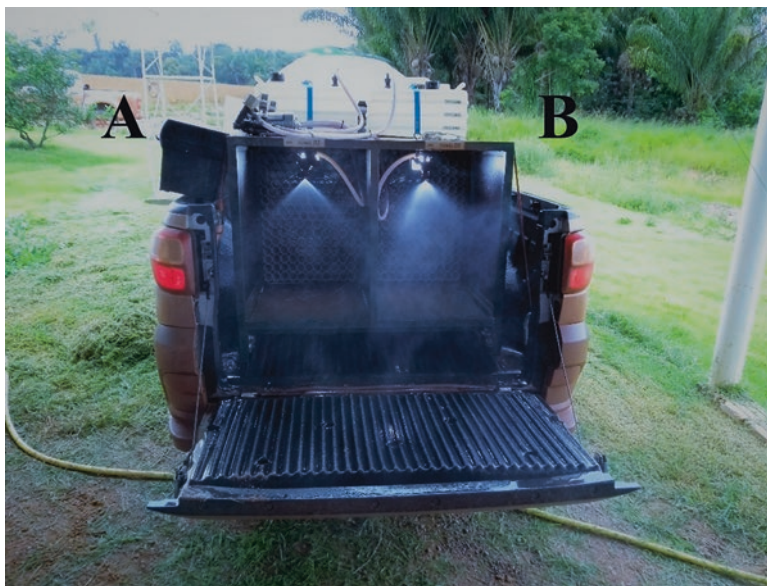
Fig. 4 Anti-drift test: (a) water with added surfactant, and (b) water without added surfactant. It is possible to verify that the cone in a is much more defined and the mixture reaches the bottom, while in b much of the mixture is lost due to drift. Photo by Maickon Balator
