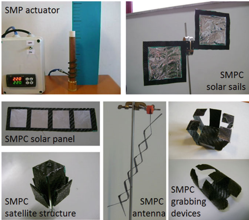
Fig. 13.3 Conceptual prototypes of actuators and space devices with SMPs and SMPCs
