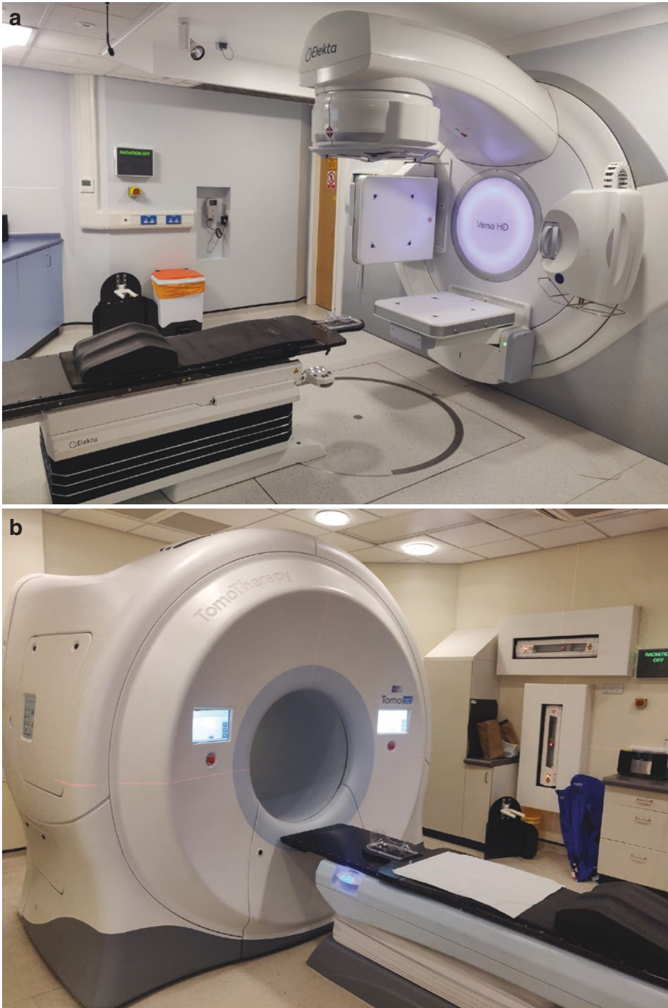
Fig. 13.1 A linear accelerator (a) and a tomotherapy unit (b) in a radiotherapy treatment room. Both deliver IMRT. The linear accelerator rotates 360° around the treatment couch, thus is able to deliver multiple beams in
