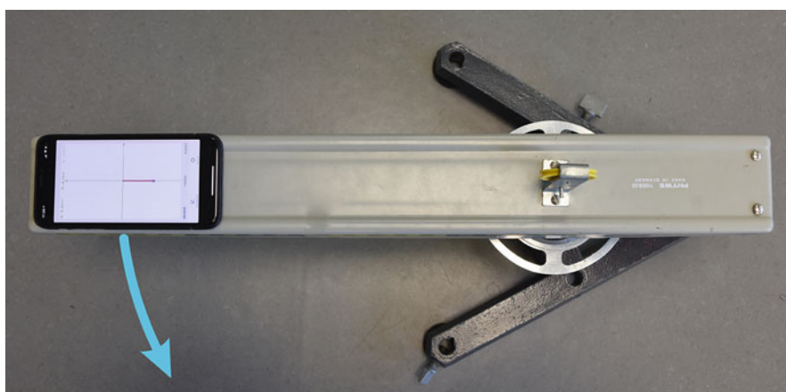
Fig. 15.4 Acceleration of a rotating iPhone
