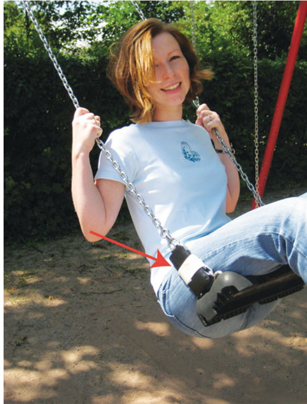
Fig. 29.3 Examination of the mathematical pendulum using a playground swing; the iPod touch is fixed to the swing with adhesive tape
