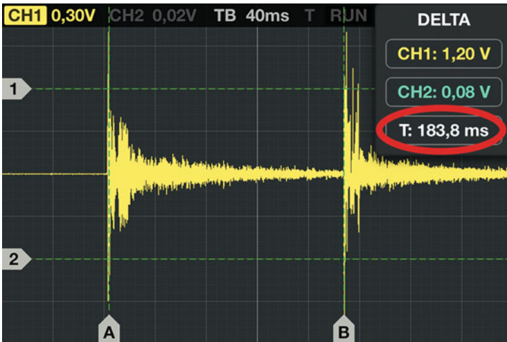
Fig. 2.2 Screen shot of the Oscilloscope App. The first peak shows the impact of the ball on the table-tennis paddle, the second one shows the impact on the wall. The time difference can be found in the app (see red circle)
