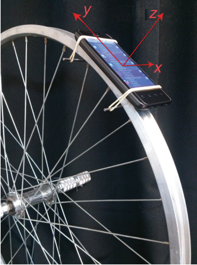
Fig. 39.1 Smartphone mounted on a bike wheel and a scheme indicating the axes orientation
