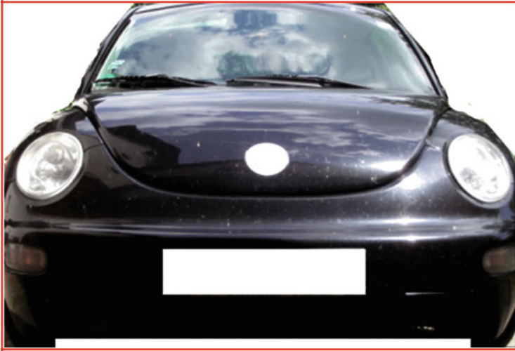
Fig. 28.1 Front view of the car. Comparing the red and white areas allows one to determine the cross-sectional area
