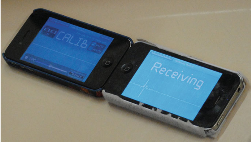
Fig. 43.1 Apparatus calibration in dual device mode: the “master” and the “reflector” devices are placed next to one another, with microphones facing each other, leaving a small gap (around 1 mm) between them, with the volume turned up on both the devices
