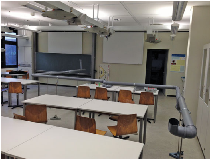
Fig. 41.2 Sound tube setup with “intermateable” drain pipes
