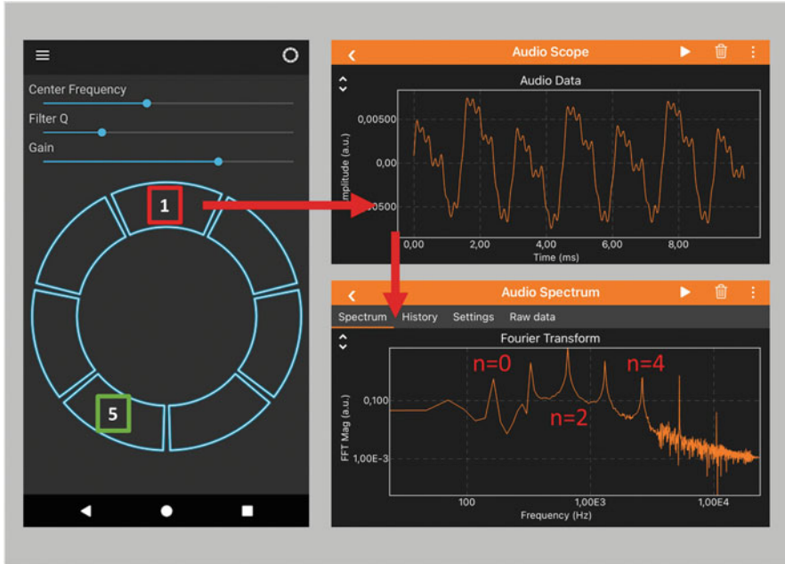
Fig. 51.2 Analysis of the waveform of the Shepard tone 1. Left: Screenshot of the app Shepard Illusion. Buttons 1 and 5 are highlighted. Right: The oscilloscopic representation reveals that the played notes are not based on a single sinusoidal wave but rather a composition of several frequencies. These can be identified by looking at the audio spectrum (FFT) of the sound. The harmonic frequency with the highest amplitude is n = 2
