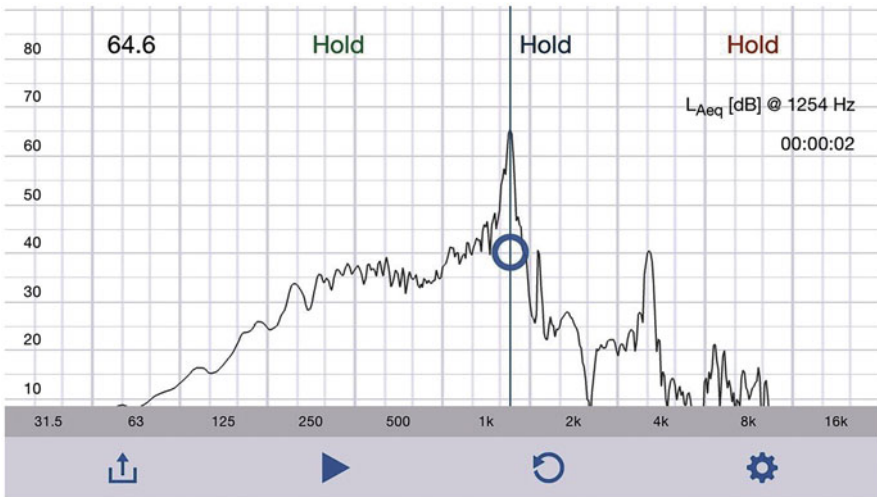
Fig. 45.2 Resonance frequency when uncorking a wine bottle (app: Spektroskop)
