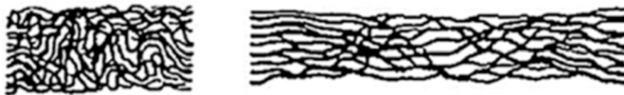
Fig. 26.1 Chains of polymer in a rubber material at different elongation
