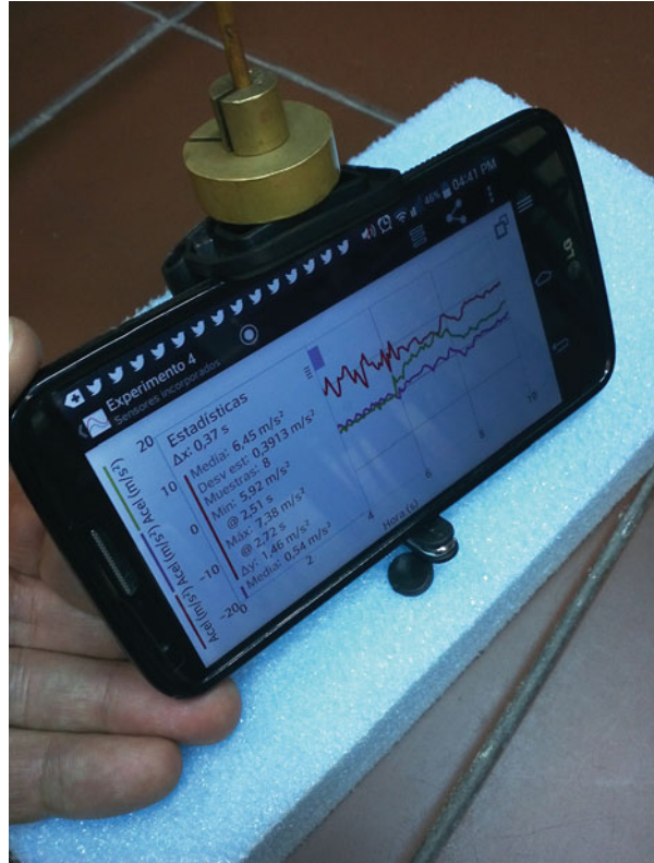
Fig. 8.3 Smartphone mounted on the support showing the Vernier app on the screen
