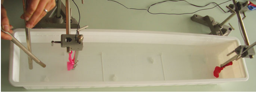
Fig. 40.4 Experiment setup to measure the speed of sound in water
