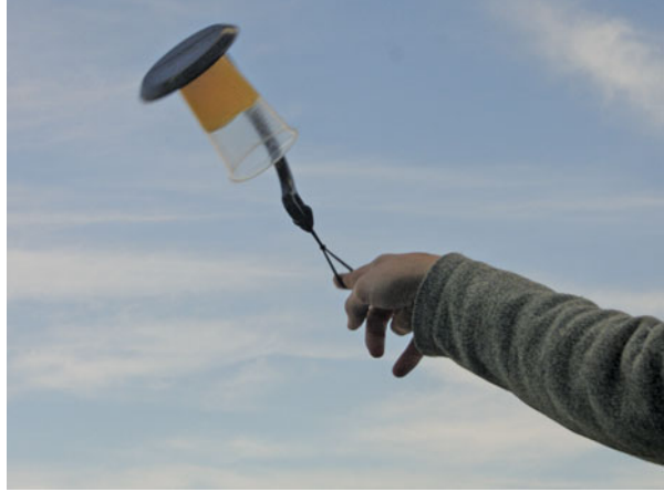
Fig. 20.1 Snapshot showing a cup on a SpillNot® giving full turns in a vertical plane; the surface of the liquid can be appreciated
