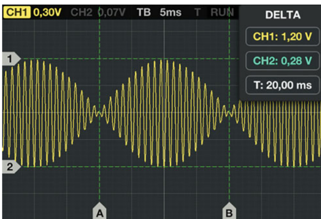
Fig. 49.3 Oscillogram of a beat
