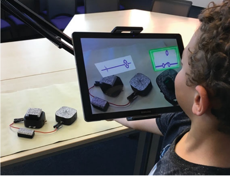
Fig. 56.2 A student exploring the tools while building an electrical circuit with the tablet setup. Once a tool is touched, the corresponding circuit symbol is highlighted
