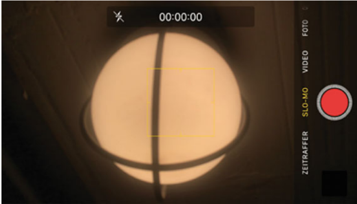
Fig. 59.3 Filming an incandescent lamp in slow-motion mode
