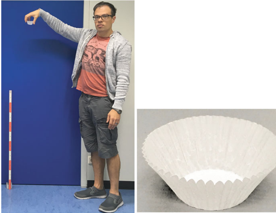
Fig. 27.1 Small paper cup used for fall experiments (right) and experimental setup (left)
