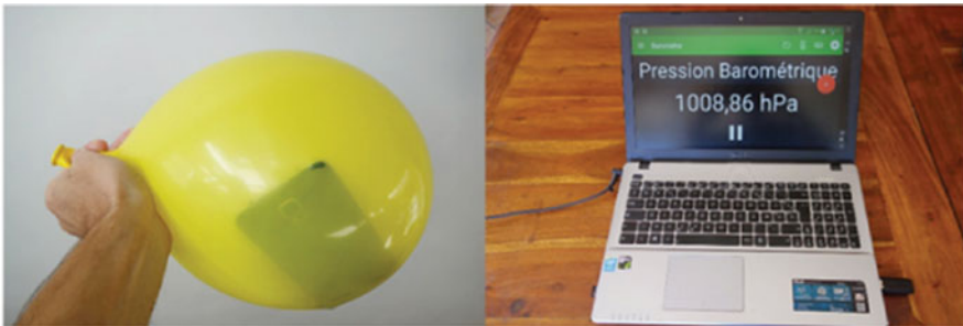
Fig. 26.4 The smartphone in a balloon! The Physics Toolbox app is controlled from the computer via Wi-Fi with the SideSync app
