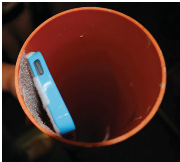
Fig. 43.2 iPhone attached to the pipe with VELCRO® brand fasteners
