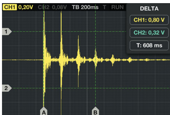
Fig. 41.4 Screenshot from the oscilloscope app; the first amplitude represents the original snapping noise, the following amplitudes are caused by following echoes
