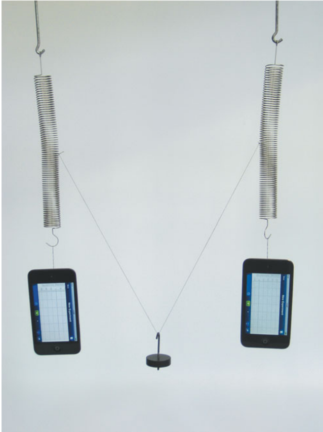
Fig. 32.3 Experiment setup for a coupled pendulum
