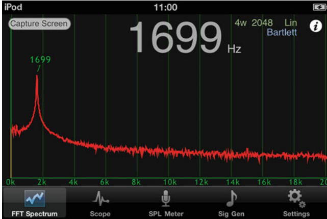
Fig. 48.2 Frequency of the tone of a 1700-Hz tuning fork
