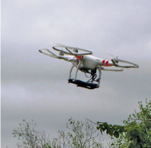
Fig. 25.4 Smartphone mounted on a DJI Phantom 2 using an armband
