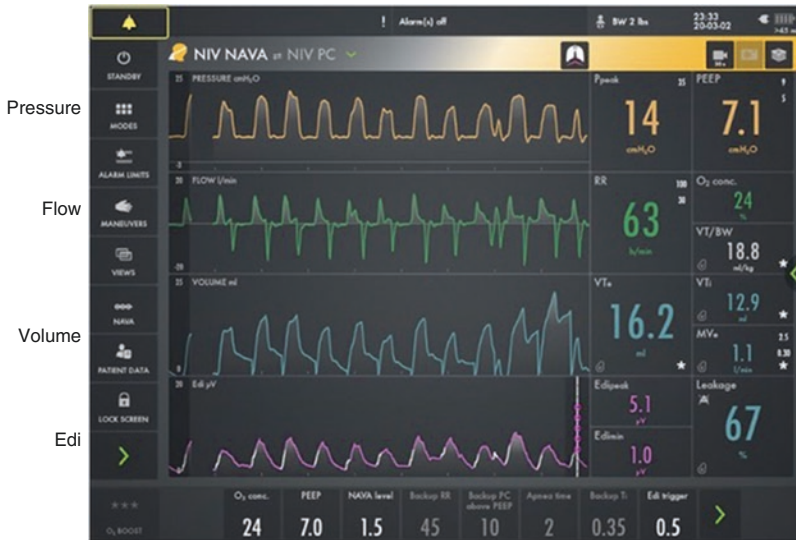
Fig. 48.3 Screenshot from the Servo-n ventilator demonstrating Edi and pressure waveforms during NIV NAVA. Bottom tracing (purple) shows the Edi waveform, with Edi peak and Edi min noted. The top tracing shows the inspiratory pressure delivered by the ventilator (yellow). The Edi and ventilator pressure waveforms during NIV NAVA demonstrate the synchrony between the patient (Edi) and the ventilator (Pvent)
