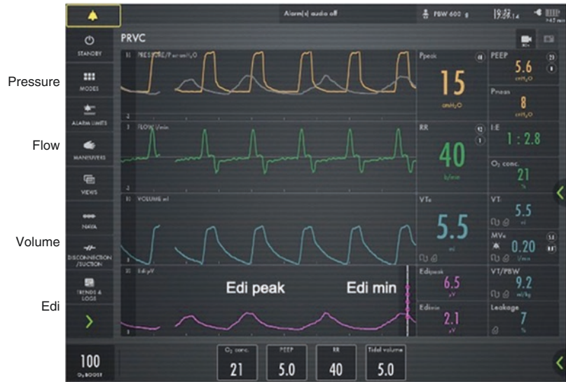
Fig. 48.2 Screenshot from Servo-n ventilator demonstrating Edi and pressure waveforms during PRVC. Bottom tracing (purple) shows the Edi waveform, with Edi peak and Edi min noted. The top tracing shows the inspiratory pressure delivered by the ventilator (yellow) with superimposed tracing of the Edi signal (light gray)
