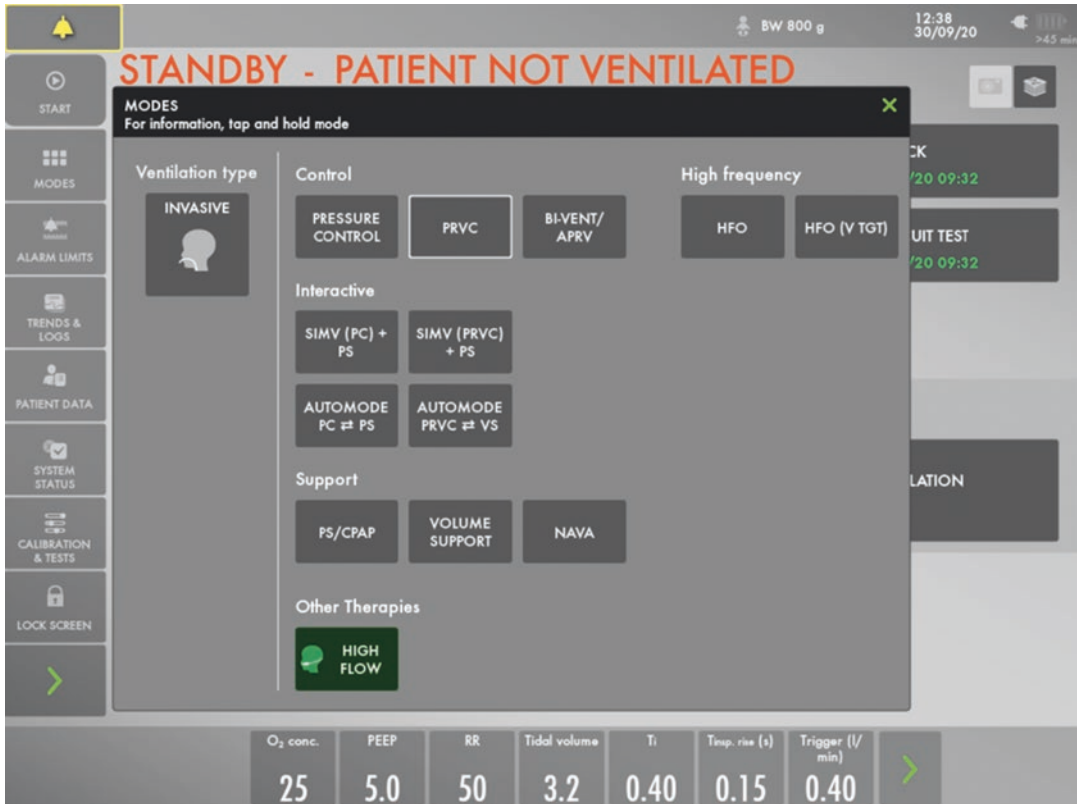
Fig. 49.2 Invasive ventilation modes and therapies available in the Servo-u/Servo-n. High flow is accessible from the invasive ventilation screen to facilitate extubation to high-flow therapy
