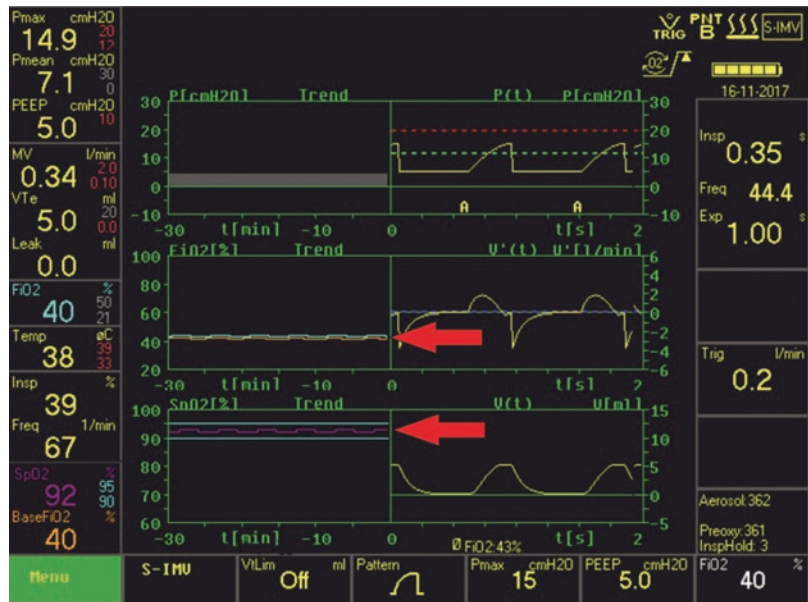
Fig. 51.6 Trend view of FiO 2 and SpO 2 (left panel, red arrows). Numeric displays on the left side show the measured FiO 2 (40%, cyan), the base FiO 2 (40%, orange), and the measured SpO 2 (92%, purple) along with the upper and lower SpO 2 target range (90–95%, cyan)
