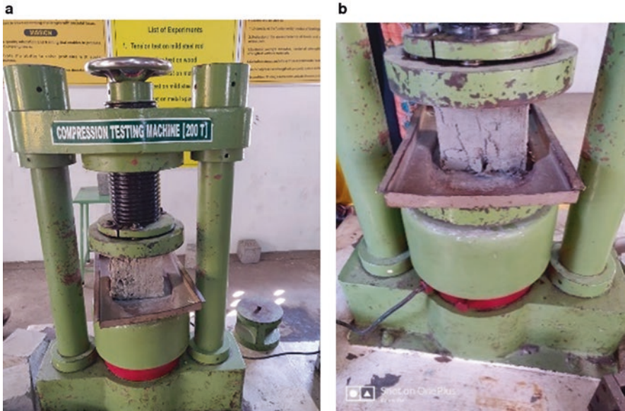
Fig. 17.4 (a) Compressive strength testing with specimens loading. (b) Compressive strength testing with failure of specimen
