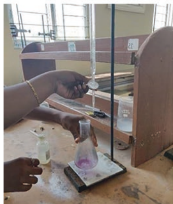
Fig. 17.5 (a) \text{CO}_2 gas produced. (b) \text{CO}_2 gas in airtight chamber. (c) Experimental setup. (d) \text{HCl} reacting with \text{Na}_2\text{CO}_3 . (e) Titration Process. (f) Balloon containing excess \text{NaOH}
