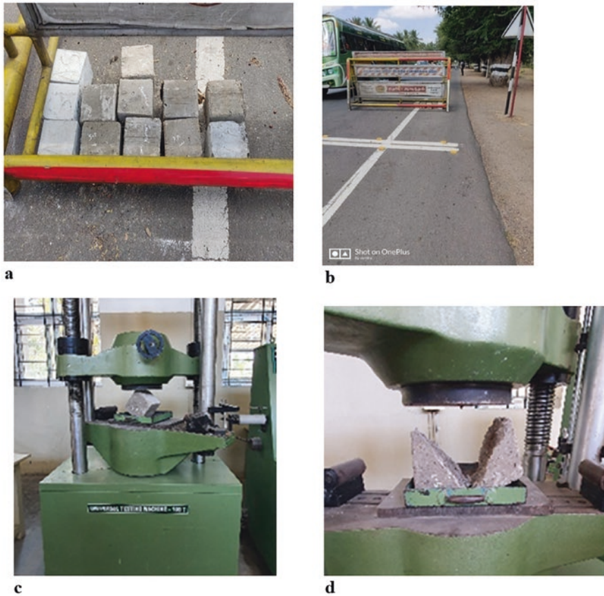
Fig. 17.6 (a) Specimens for CO 2 open atmosphere. (b) Specimens for CO 2 atmosphere. (c) Splitting of specimen. (d) Splitting of specimen
