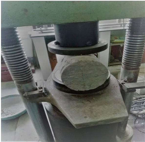
Fig. 40.5 Split tensile strength of cylinder performed by using universal testing machine
