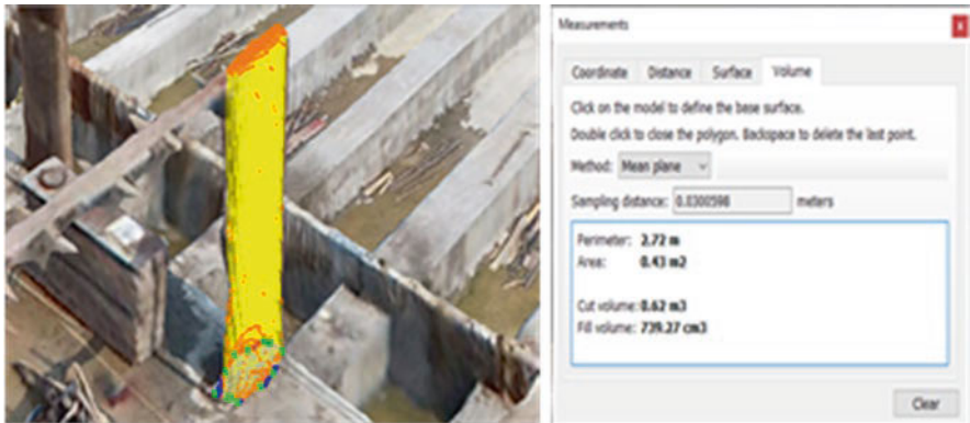
Fig. 57.15 volume of concrete for a column calculated from the 3D model from context capture (Phase II)
