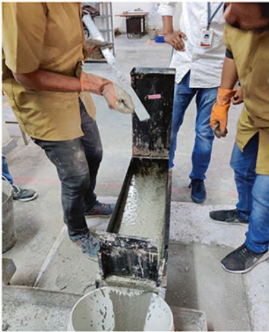
(ii) Measuring V-Funnel flow time
