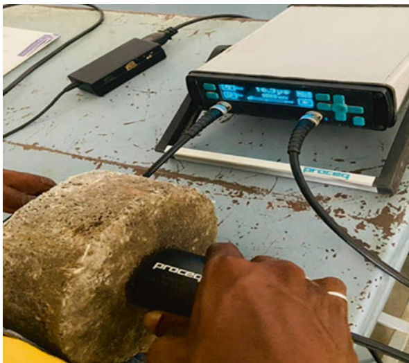
Fig. 44.8 Ultrasonic pulse velocity testing
