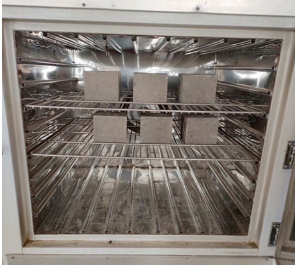
Fig. 38.5 Curing of specimen at 60 °C in hot air oven
