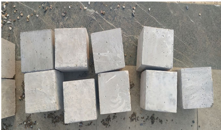
Fig. 11.1 Demolded cube specimens. (Source Author)
