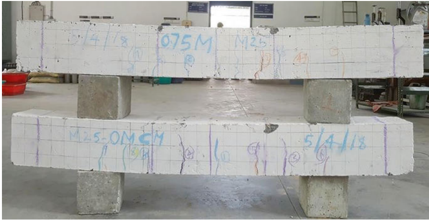
Fig. 46.11 Flexural cracks in the beam after testing
