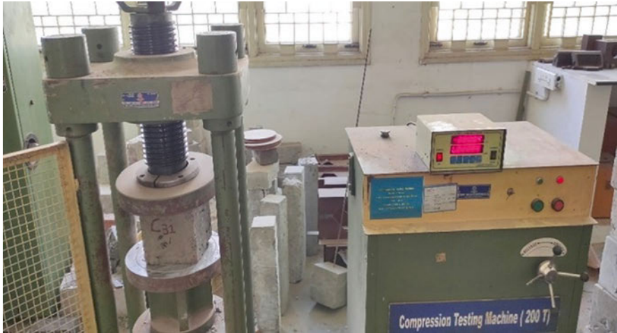
Fig. 40.2 Compression test of cube performed by using universal testing machine
