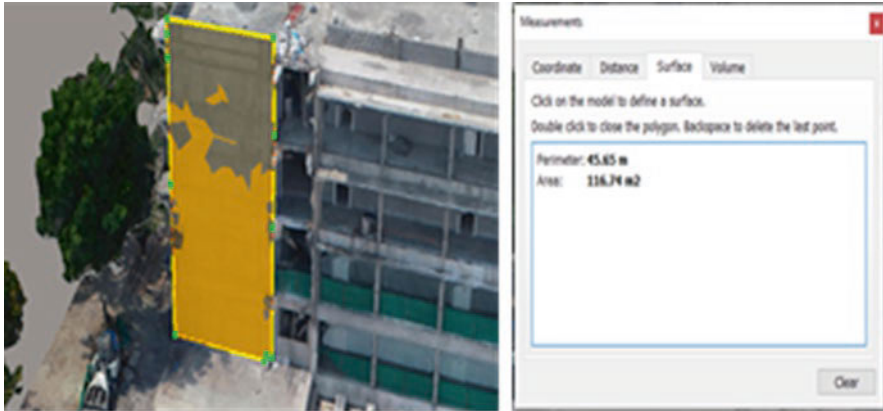
Fig. 57.16 Area of wall to be plastered Calculated from the 3D model from context capture (Phase II)
