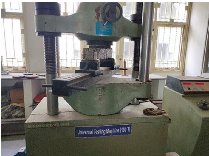
Fig. 40.7 Flexural strength of prism performed by using universal testing machine
