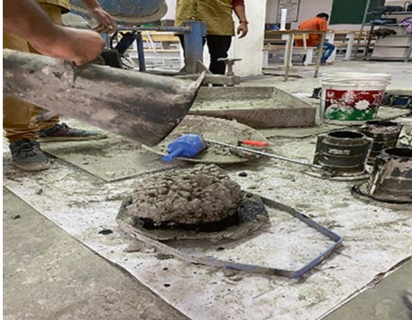
Fig. 45.1 Slump cone test
