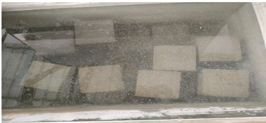
Fig. 11.2 Concrete cubes in curing. (Source Author)
