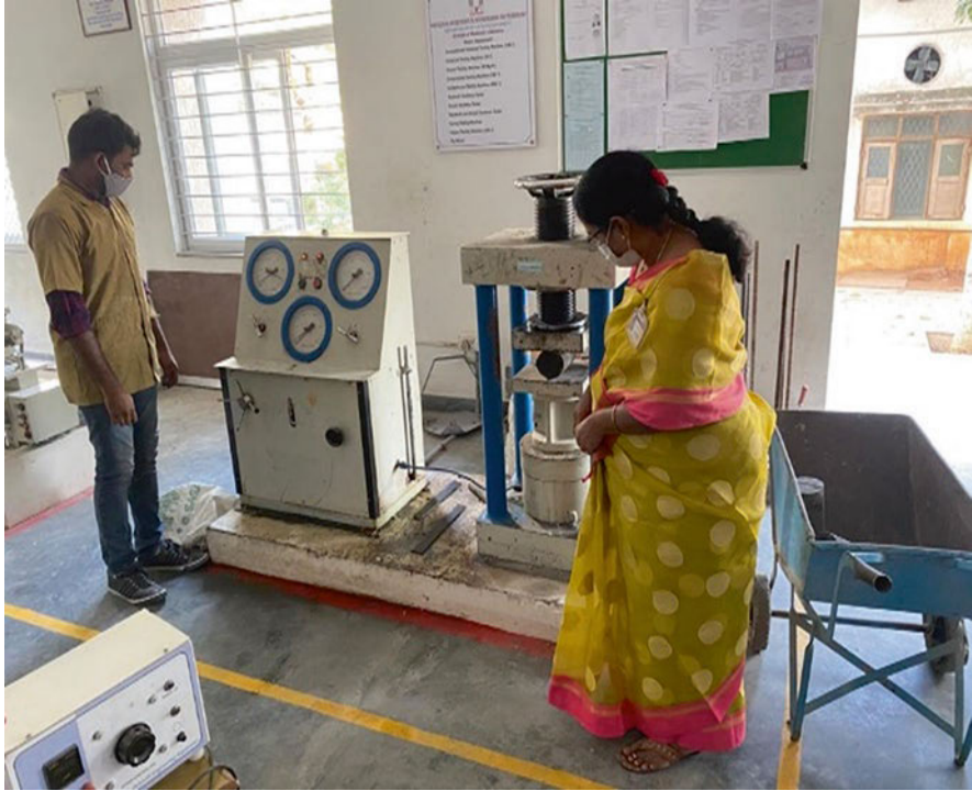
Fig. 45.5 Cylinder specimen placed in split tensile testing machine
