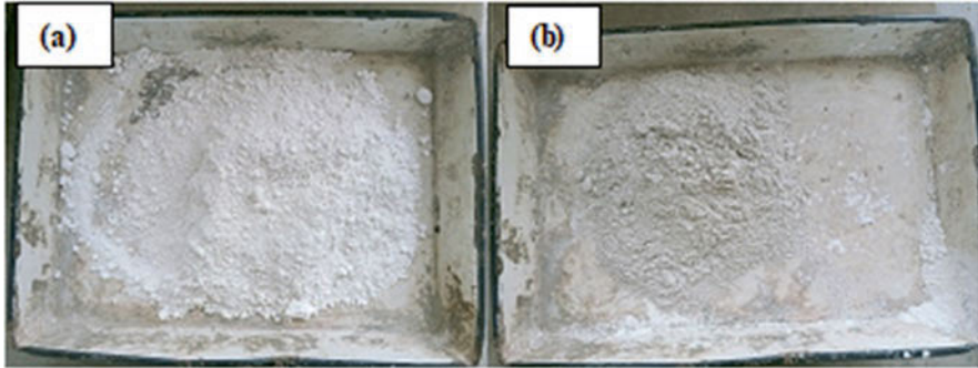
Fig. 30.1 (a) Calcined clay (b) GGBS
