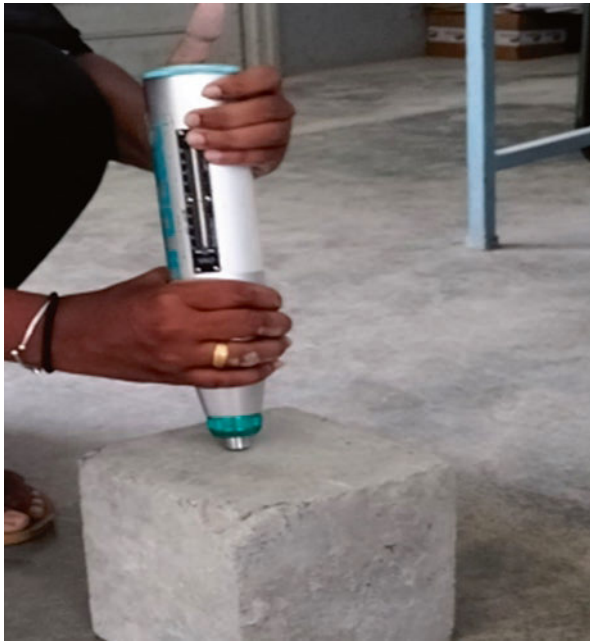
Fig. 44.9 Rebound hammer testing
