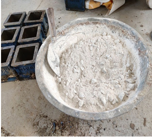
Fig. 38.2 Dry mixture of Geopolymer concrete
