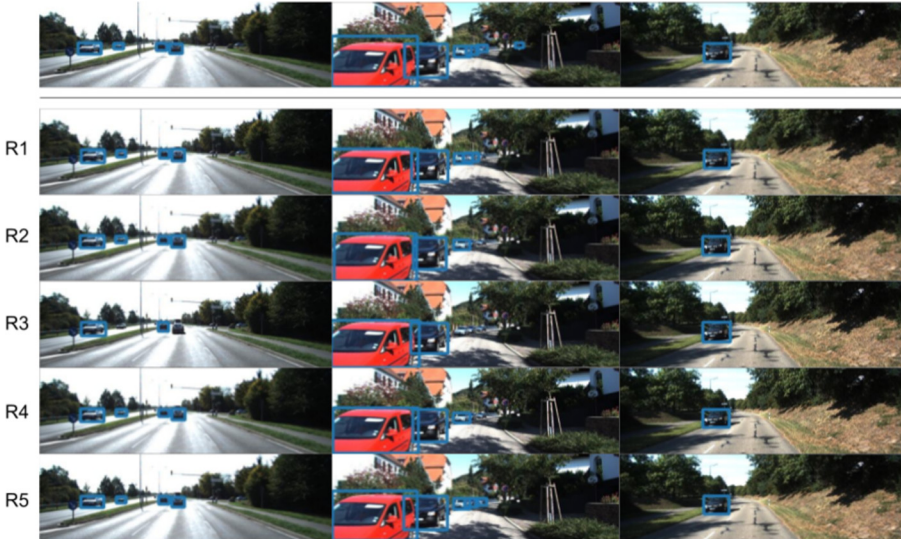
Fig. 4. The ground truth is shown above the line and predictions on images from the KITTI dataset, generated by the different models, under the line. The models from top to bottom are: no TL ( Base ) (R1), feature adaptation (R2), cycleGAN (R3), feature adaptation with cycleGAN (R4), and Oracle (R5).
