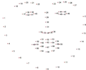
Fig. 1. View over the 68 coordinates of the face marker in the iBUG 300 W data set [11].
