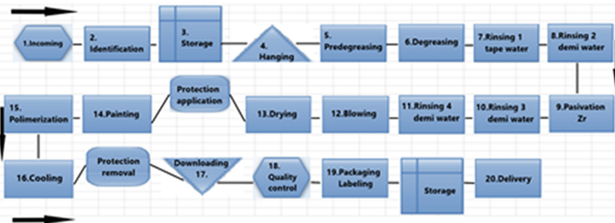
Fig. 1. The process flow diagram in the electrostatic field powder paint.
