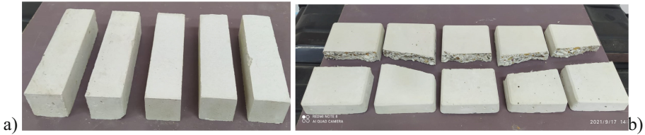
Fig. 1. Images with five micro-concrete with nano-TiO 2 : a) before testing; b) after testing
