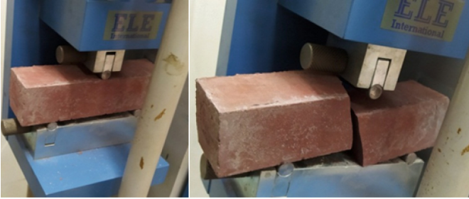
Fig. 4. Alkali-activated geopolymer samples during flexural strength test.
