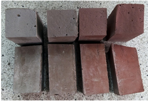
Fig. 5. Alkali-activated geopolymer samples after flexural strength test.
