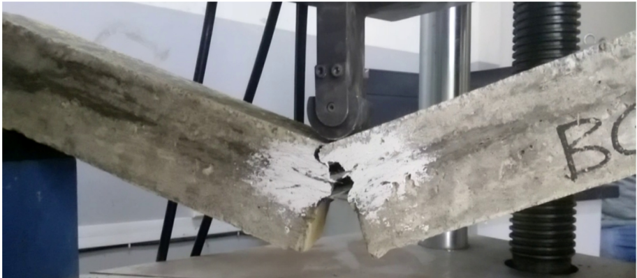
Fig. 14. Crack patterns at 0.6% glass fiber addition for C20/25 design grade concrete just before failure.
