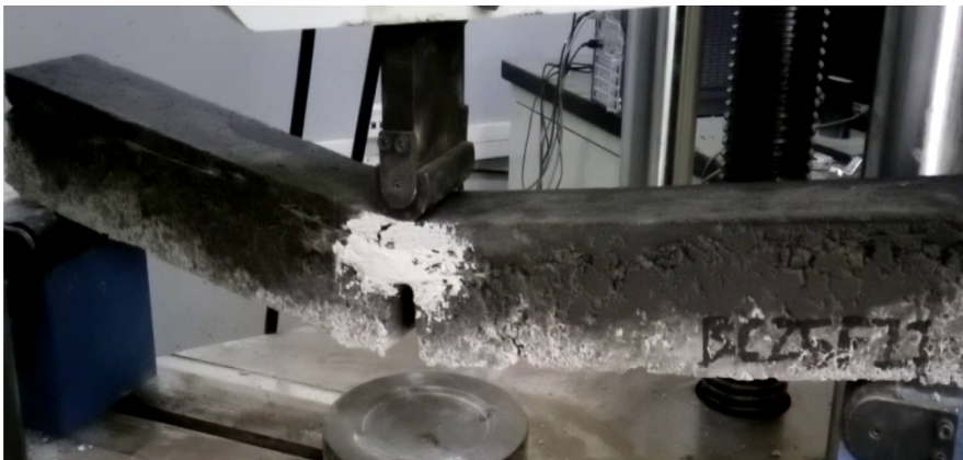
Fig. 12. Crack patterns at 0.2% glass fiber addition for C20/25 design grade concrete just before failure.
