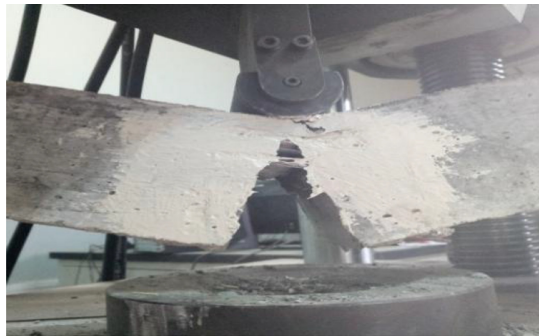
Fig. 10. Crack patterns at 0.4% glass fiber addition for C25/30 design grade concrete just before failure.
